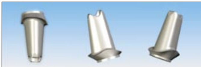
Fig. 2: Virtual abutment created through computer-aided design (CAD) can be evaluated for proper morphology prior to milling process.
